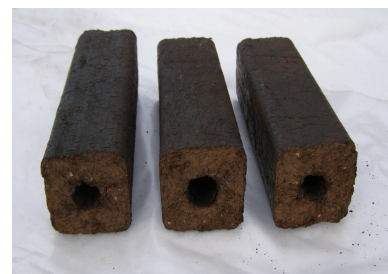
Briquette 50x50x250÷300MM, with hole in centre
